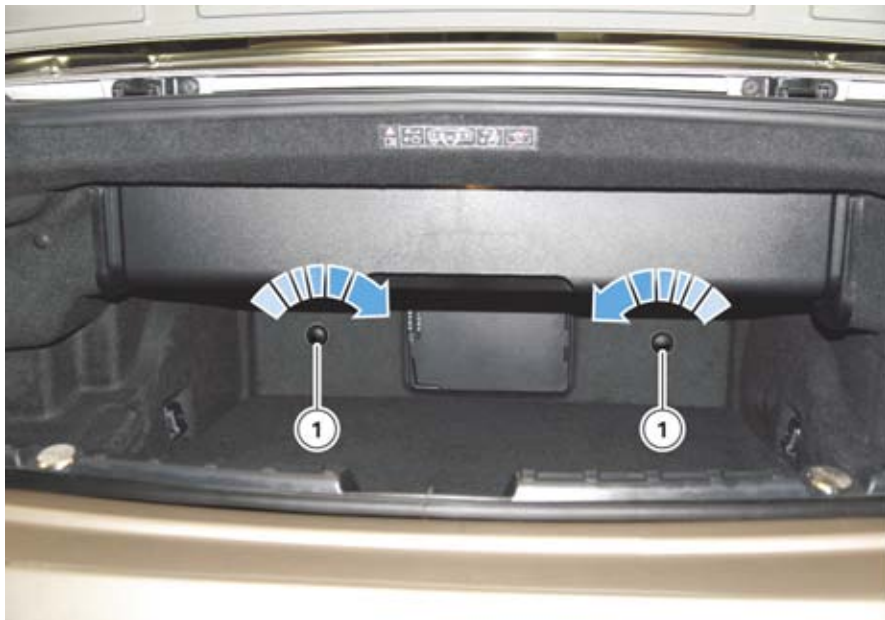
F12 Service activation of roll-over protection system
